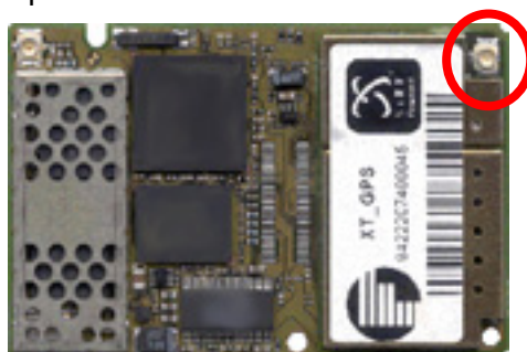
Figure 35: GPS antenna connector (U.FL-R-SMT connector)
