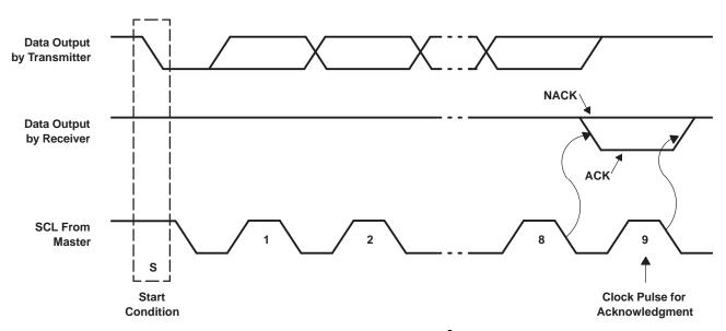
Figure 3. Acknowledgment on I<sup>2</sup>C Bus
