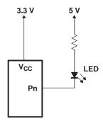
Figure 17. Device Supplied by Lower Voltage
