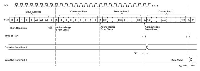
Figure 6. Write to Output Port Registers
