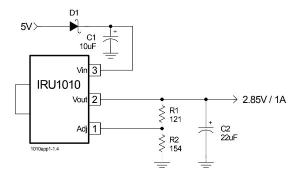
Figure 1 - Typical application of IRU1010 in a 5V to 2.85V SCSI termination regulator
