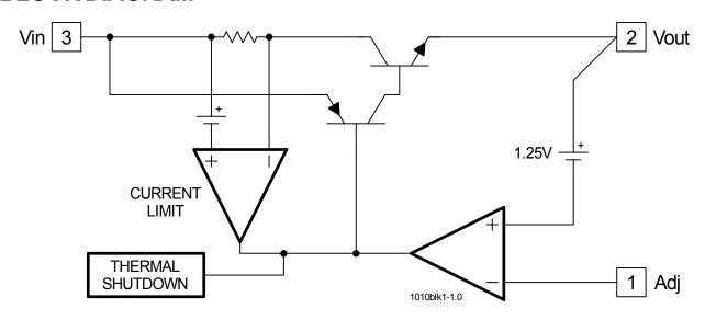
Figure 2 - Simplified block diagram of the IRU1010
