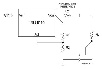
Figure 4 - Schematic showing connection for best load regulation
