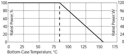
Derating (thermal resistance): 2.86W/°K (0.35°K/W).
