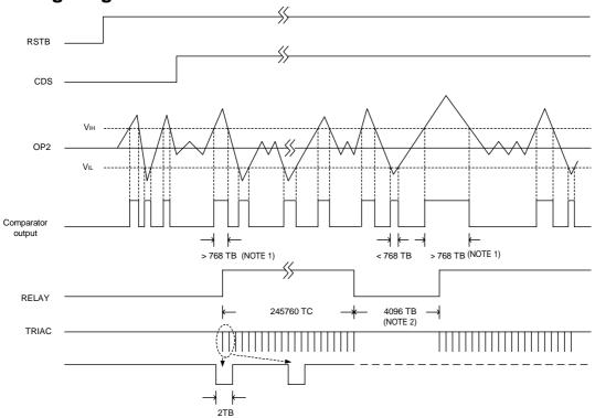
NOTE: (—)COMPARATOR OUTPUT SIGNAL SHOULD BE LARGER THAN 768 TB CYCLE, THEN THE SYSTEMS IS ACTIVATE, IF NOT, IT WILL DEACTIVATE.
