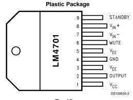
Top View Order Number LM4701T See NS Package Number TA9A For Staggered Lead Non-Isolated Package Only a 9-Pin Package
