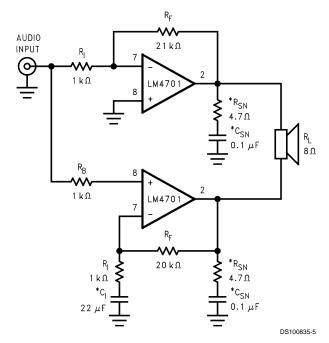
FIGURE 2. Bridged Amplifier Application Circuit
