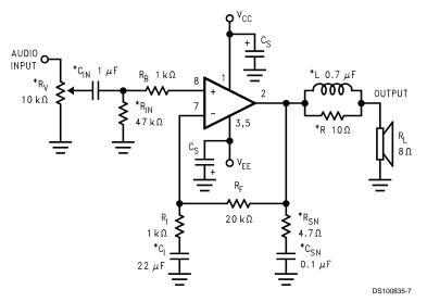
FIGURE 4. Auxillary Amplifier Application Circuit
