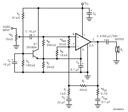
FIGURE 3. Single Supply Amplifier Application Circuit
