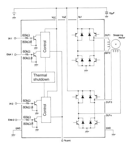
Note: As long as the voltages applied to  $V_{CC}$ ,  $V_S1$ ,  $V_S2$ , ENA1, ENA2, IN1, and IN2 are within the limits set by the absolute maximum ratings, there are no restrictions on the relationship of each voltage level in comparison with the others (regarding which is higher or lower). (ex.  $V_{CC} = 3$  V,  $V_S1$ , 2 = 2 V, ENA = IN = 5 V)
