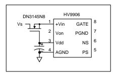
This method limits the  $+V_{IN}$  voltage to  $V_{DD}$  +  $V_{GS(OFF)}$  of the depletion MOSFET for all input voltages and in fact raises the maximum allowable peak input voltage to the breakdown voltage rating of the depletion MOSFET. The worst-case power dissipation in the HV9906 is now given by the equation
