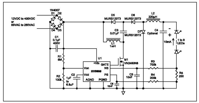
This circuit provides a constant average current output, which may be used to power LED lamps. The circuit maintains a constant average current and the value of C4 capacitor controls the peak-to-peak ripple, which decreases with increasing capacitor value.
