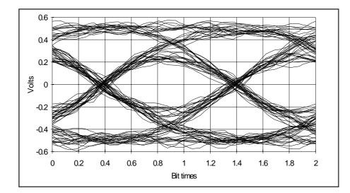
Fig.14 Effect of Noise (BT = 0.3) (noise bandwidth = 2 x bitrate; S/N = 25dB)
