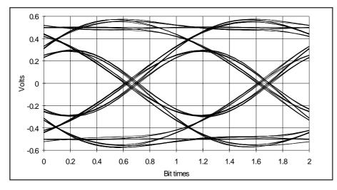
Fig.12 Effect of Poor Channel Amplitude and Phase Response
