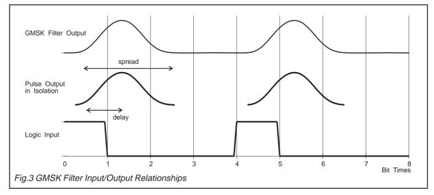
True GMSK transmission, in radio, is achieved when the 'data' output of the Gaussian filter is passed through an FM modulator having a continuous phase response, with the peak deviation being set to half of the applied bit rate.
