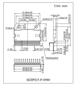
Note) The package of this product will be changed to lead-free type (HZIP025-P-0980B). See the new package dimensions section later of this datasheet.
