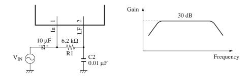
The gain can be reduced by inserting a resistor Rf in series with the electrolytic capacitor at Pin6.
